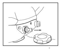
**NOTE:** the choke is on "FULL" when the knob is pulled out all the way. The choke is "OFF" when the knob is pushed in. This is a variable choke and can be adjusted gradually, depending on how much choke is needed for starting.
